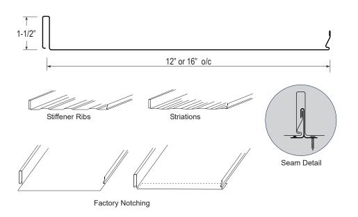
TBC-TRULOC is the #1 choice for standing seam metal roofing in light commercial or residential applications. The 1-1/2" height and continuous positive seam engagement offer exceptional strength and weathertightness. The separate galvanized clip allows the panel to thermally expand & contract, which is critical with longer length applications.
