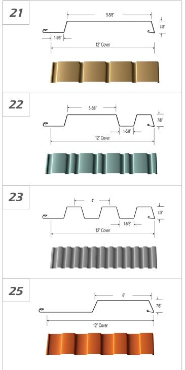
\* Profiles shown on front page with fastening flange and back page with clip seam.
