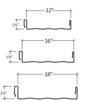
One of the most versatile architectural metal panels available today, LokSeam® by ABC, is a snap-together, concealed fastener, standing seam roof system with a 1¾" tall vertical rib, for use on roofs with a minimum slope of 3:12. Available in 12-inch, 16-inch and 18-inch widths, LokSeam® panels can be installed over open framing or a solid substructure and are capable of transitioning from roof to fascia with the use of a rib cover and does not require a solid substructure for support.
