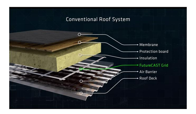
Above: The FutureCast Grid is installed on the lowest possible layer of a conventional roof assembly in order to track moisture that has worked its way down through the protection layers or detect condensation from construction and operation activity which has been sealed inside the assembly.
