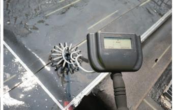
Leaks and penetrations are found on a roof membrane after the first scan
